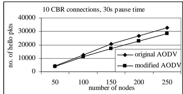
Figure 5: No. of hello packets transmitted vs number of nodes
