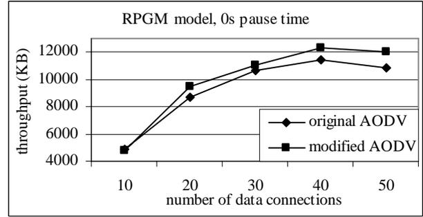
Figure 14: Throughput vs number of data connections
