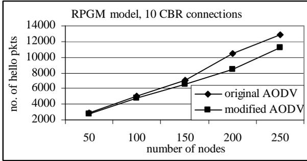
Figure 13: No. of hello packets transmitted vs number of nodes
