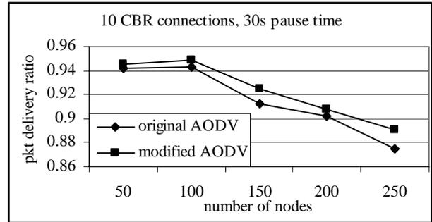
Figure 3: Packet delivery ratio vs number of nodes
