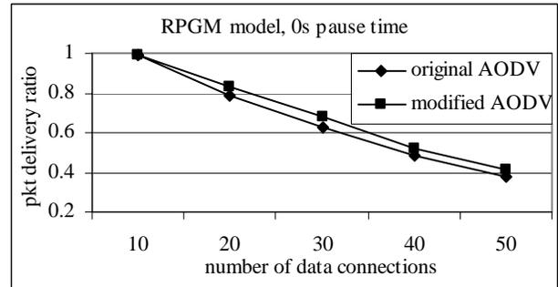
Figure 15: Packet loss ratio vs number of data connections
