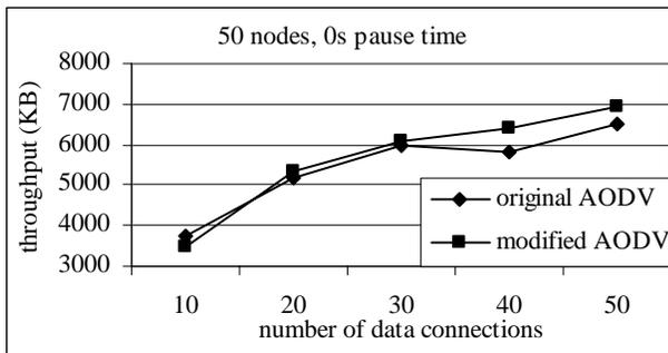
Figure 6: Throughput vs number of data connections
