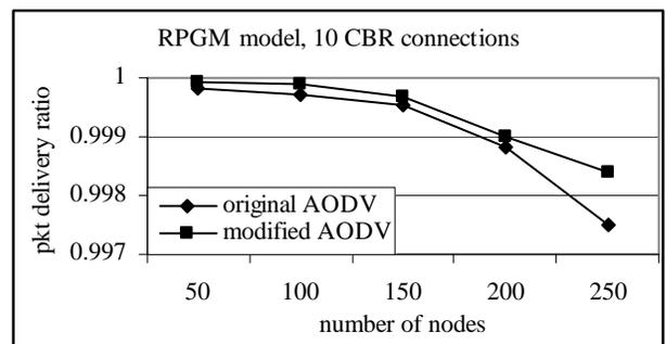
Figure 11: Packet delivery ratio vs number of nodes
