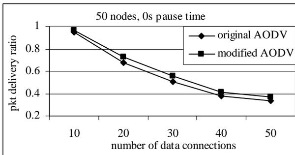
Figure 7: Packet delivery ratio vs number data connections
